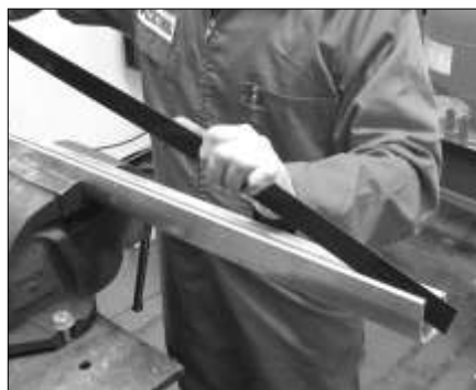
Fitting new scraper blade to extrusion
