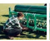
Attach tow cable to tractor and Double-Quick.
