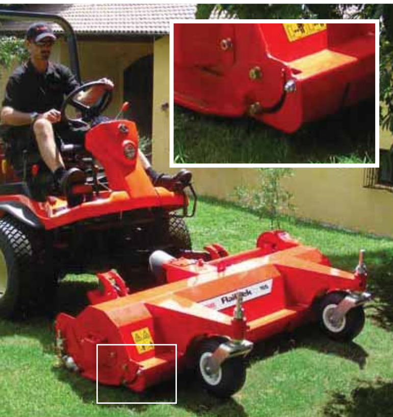
For short grass cutting the Converter is set in the closed position
