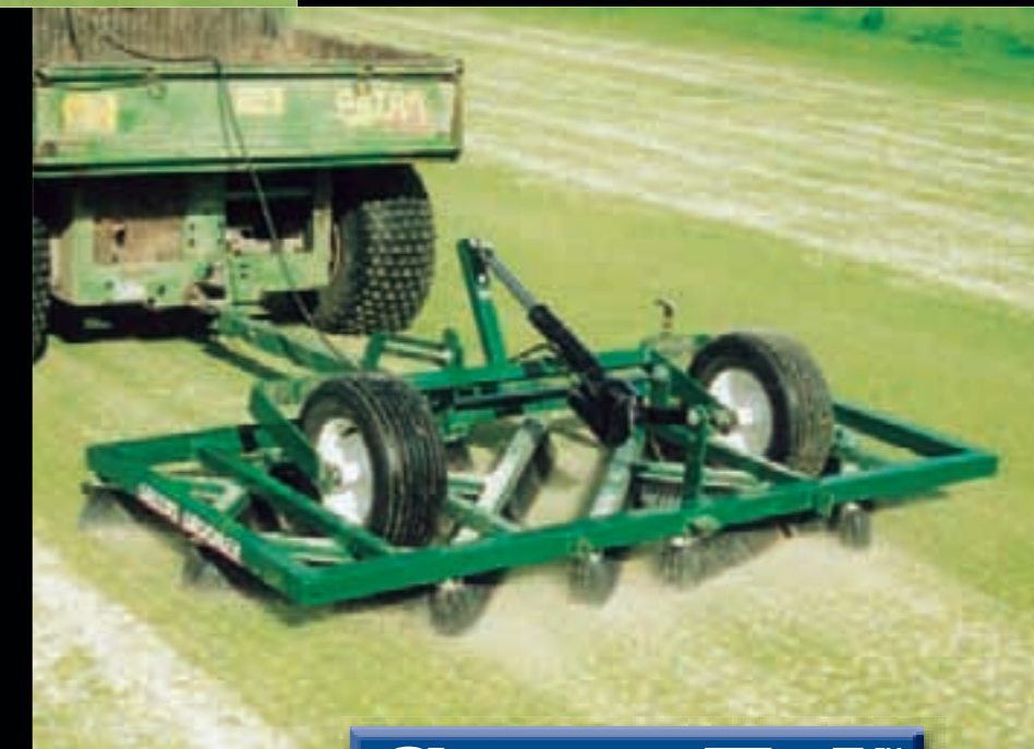
The Greens Groomer works the sand down into the surface between the blades of grass.
