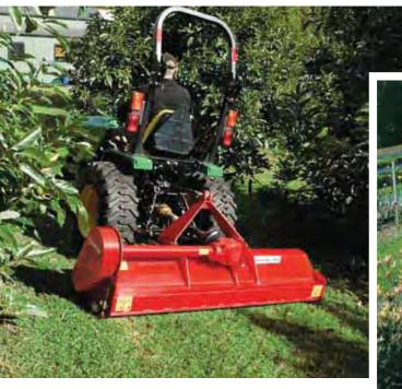
(A) Three point linkage mounting Dual category linkage pins.
