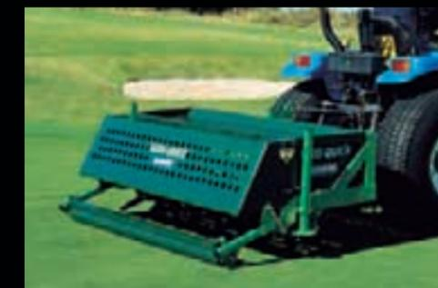
The Aero-Quick's 5' (1.5m) working width covers the track of most compact tractors and utility vehicles.
