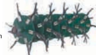
**SOLID TINER** - The round 4" tines spike neat holes in outfield turf which help prevent clay soils cracking in dry weather. Not recommended for use on greens, unless well rooted.
