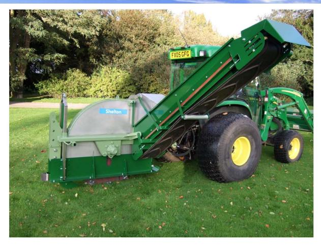
Designed for installing pipes and secondary drainage on sportsturf.
