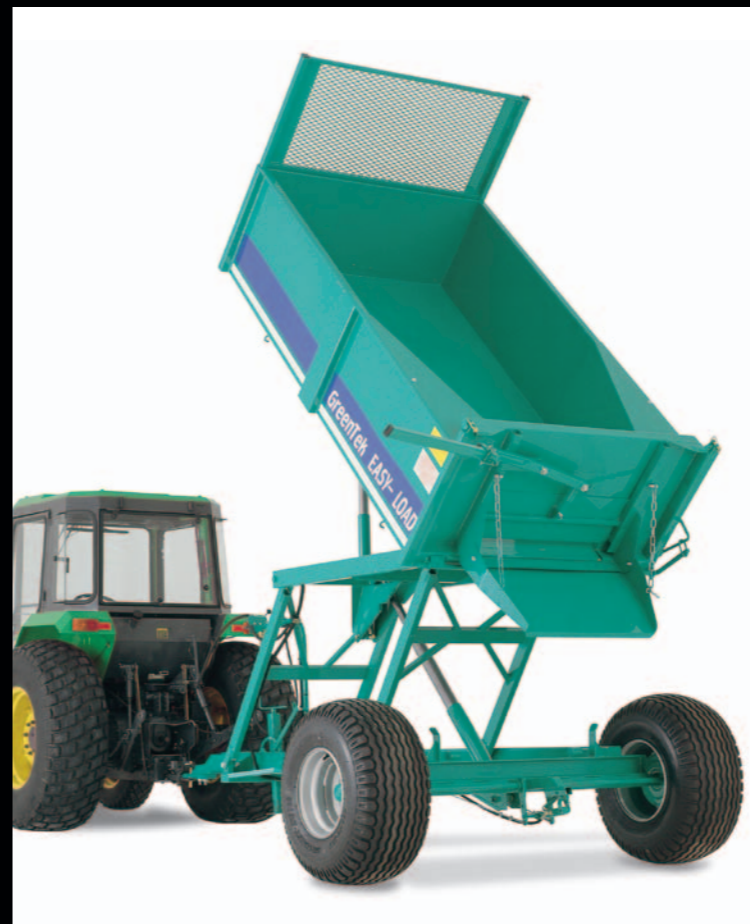
Wheels spaced outside body width provide extra stability for high tipping.
