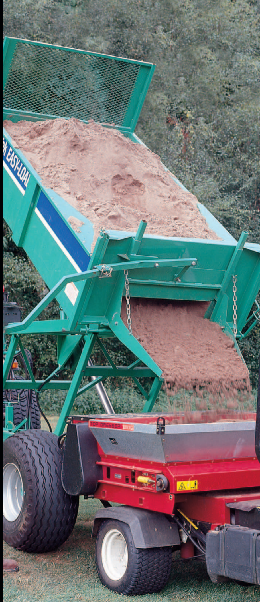
Wheels spaced outside body width provide extra stability for high tipping.
