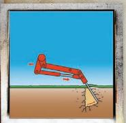
Verti-Drains adjustable parallelogram design shatters the soil, and also allows for clean Coring, on all models.
