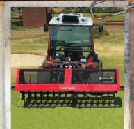
The Level-Spike is built tough and can be operated at speeds of 8.7mph (14 kmh) or more. The choice of available widths enables the customer to match the machine to their tractor and their specific requirements. There is an exceptionally wide range of knife options. There is an optional hydraulic weight transfer system which utilizes the tractor's hydraulics to force the tines into the ground providing maximum aeration and drainage.
