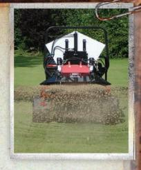
The Rink DS 800 is a topdresser with dual spinners with a spread pattern variable up to 10 m. The operation of the belt and spinners can be done from the tractor seat, by switching the hydraulic lever. No unnecessary drop of material takes place between stopping and operation, since the material release gate automatically closes when the belt is stopped. The spinner disks have been designed in a way that they will handle wet material very well.
