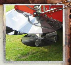
The Rink DS2000 Disc Spreader is a large top-dresser with dual spinners and a variable spread pattern of up to 40 feet. Its total capacity is 2.6 cubic yards and it can cover a lot of turf in a short time. The high floatation tires have a lighter footprint than the most competitors and the state of the art spinners leave an even spread pattern that is unequaled.
