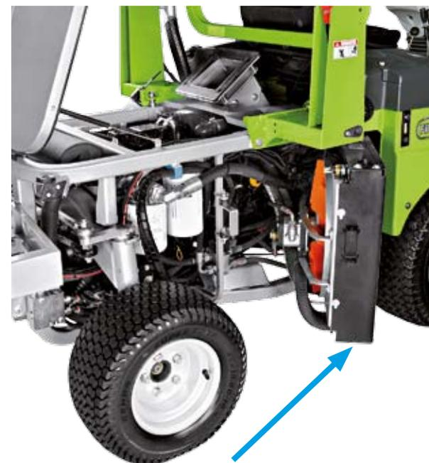
The radiator opens outward to facilitate inspection and cleaning and it is equipped with an automatic system which reverses the rotation of the fan, in order to keep clean the whole surface of the radiator grid, and to guarantee constant control of the temperature. If needed, this operation can also be carried out manually by the operator.
