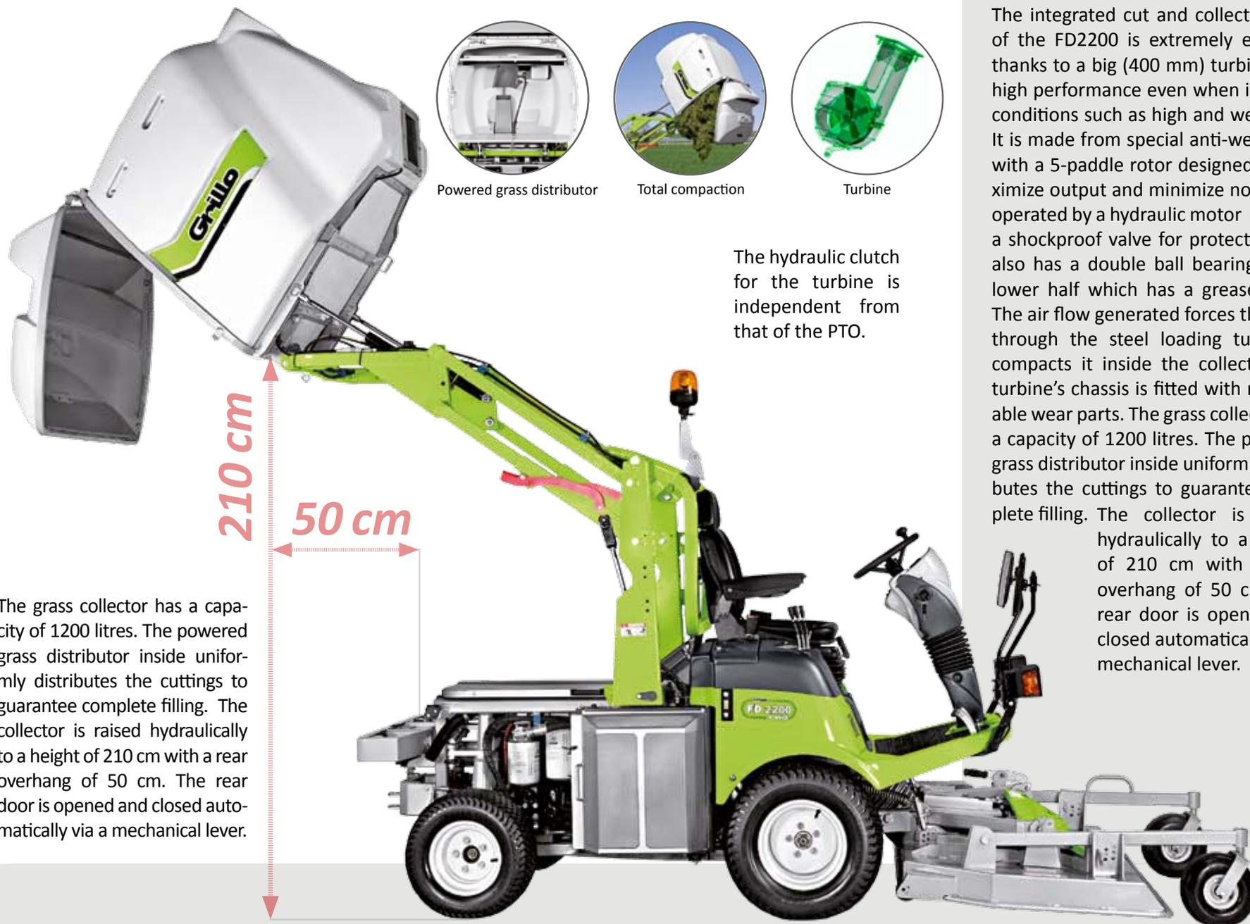
The grass collector has a capacity of 1200 litres. The powered grass distributor inside uniformly distributes the cuttings to guarantee complete filling. The collector is raised hydraulically to a height of 210 cm with a rear overhang of 50 cm. The rear door is opened and closed automatically via a mechanical lever.
